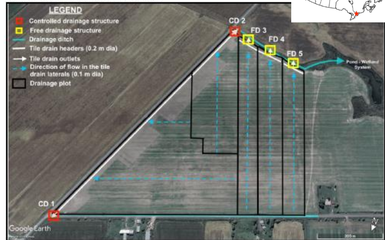
Fig. 1. Location of drainage structures with direction of flow in the tile drain laterals shown.
