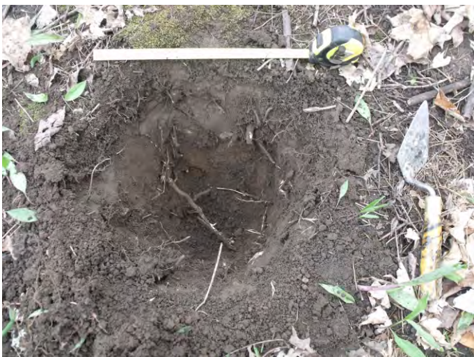
Plate 9: TP 2 showing silt loam topsoil over a cobble layer, facing N (Photo 3346).
