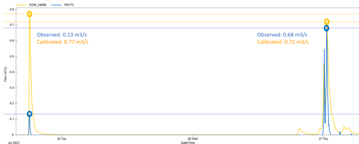
Figure 4-5. FM175 Observed Flow (Blue) and Modeled Flow (Yellow) Comparison
