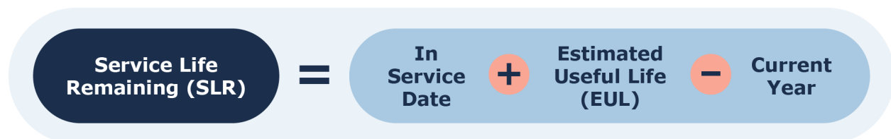
Figure 2: Service Life Remaining Calculation
