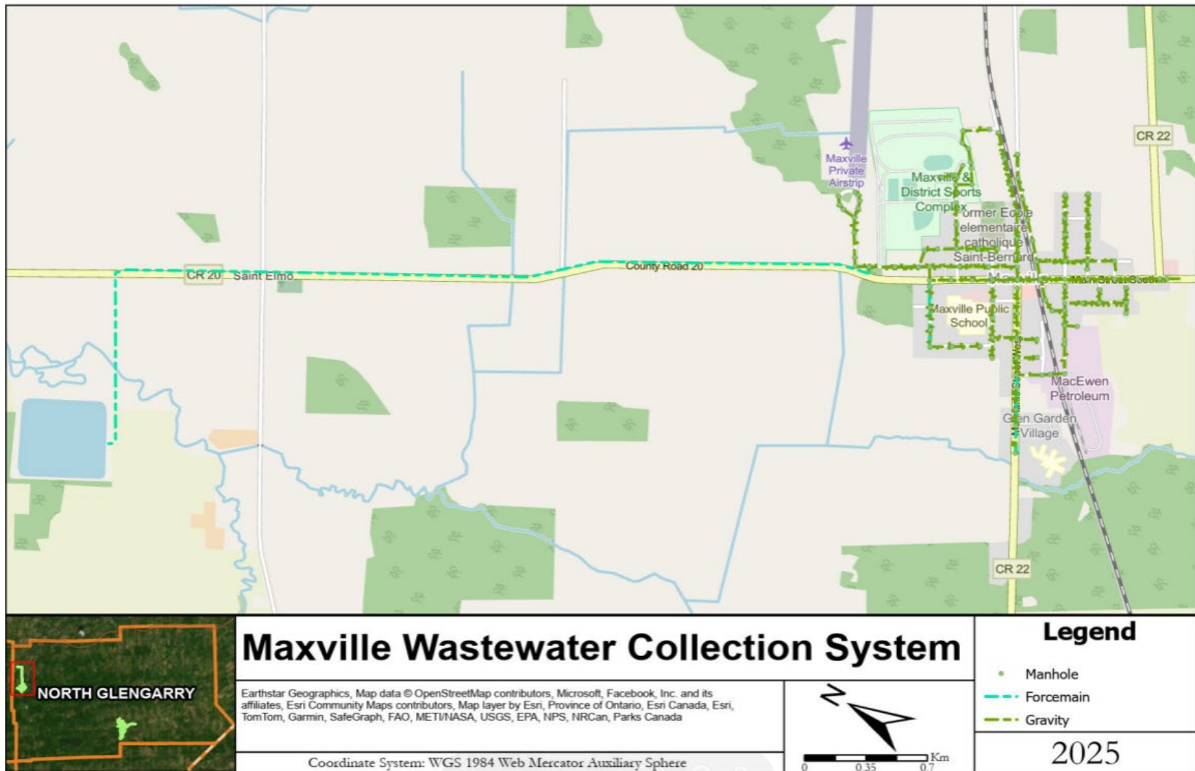
Figure 17 Maxville Wastewater Collection System Layout
