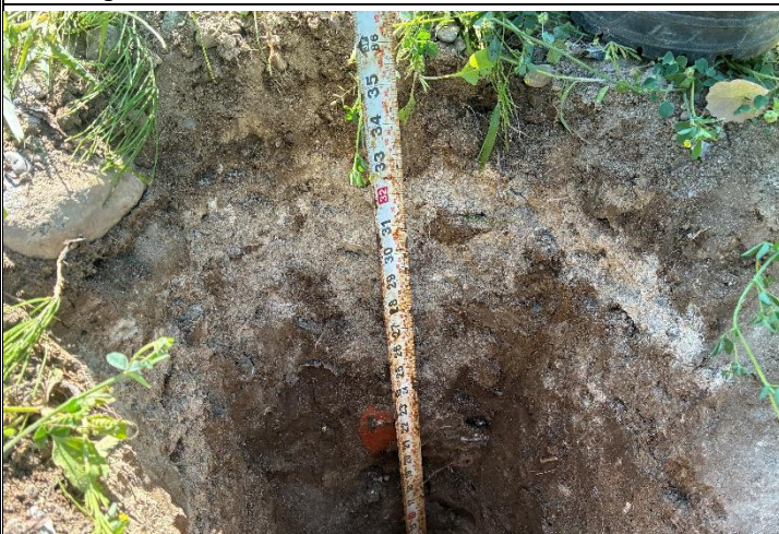
17. Test hole 2 excavated for inspection of mantle material and collection of native soil
