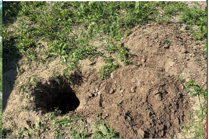
14. Test hole 1 excavated for collection of filter base material
