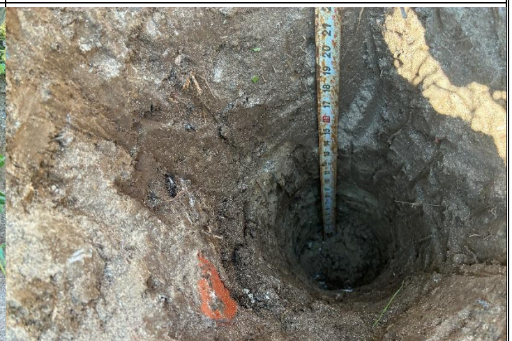
18. Base of test hole 2. No ground water observed.
