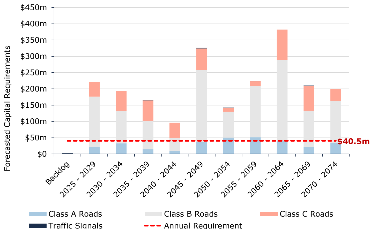
Figure 27 Forecasted Capital Replacement Needs: Road Network 2025-2074
